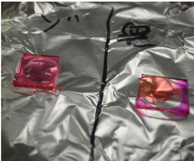
Figure 6. Picture of two samples. Since water was dropped on the film on the right side, the film came off the glass substrate. Another hybrid film on the left side without water was not destroyed, although it exposed in air for the same duration.
